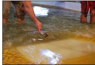
Physical modeling of Calgary Bow River Weir Project
