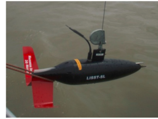
Laser-based in-situ grain size measurements, Fraser River Estuary, Vancouver, BC
